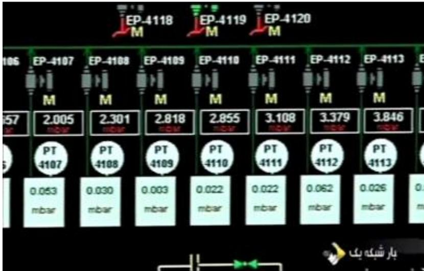
The monitoring screen for the Cascade Protection System, shown above, shows the basic piping, valves, and pressure sensors of the cascades. Red piping (upper display area) signifies the feed header. Blue piping (lower left display area) signifies the product take-off, white piping (lower right display area) signifies the tails take-off, and green piping (upper display area, extending down left and right at the display borders) the pressure normalization and dump system.
