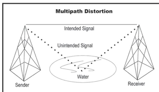
Multi-path distortion occurs in outdoor deployments where a signal traveling to the receiver arrives from more than one path. This can occur when the radio wave traverses over water or any other smooth surface that causes the signal to reflect off the surface and arrive at a different time than the intended signal does.
