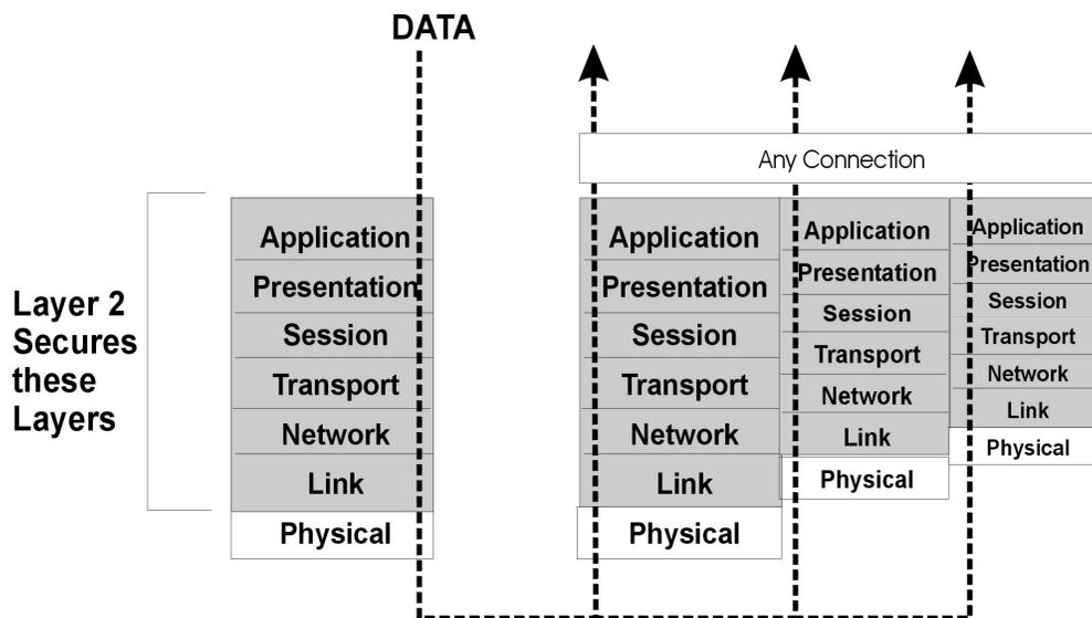
The Wi-Fi Alliance has taken work done by the IEEE 802.11TG and adopted key portions to create a new standard called Wi-Fi Protected Access (WPA). WPA is an industry standard for providing strong link layer security to WLANs, and supports two authenticated key management protocols using the Extensible Authentication Protocol (EAP). WPA also requires data frame encryption using TKIP (Temporal Key Integrity Protocol) and message integrity using a Message Integrity Check (MIC) called Michael.
