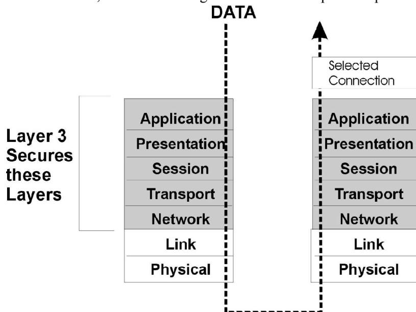
IPSec is the standard network layer security protocol, and provides a standard and extensible method to provide security to network layer (IP) and upper layer protocols such as TCP and UDP. It is used
