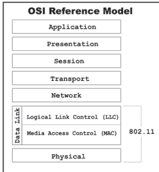
As with any of the other 802 networking standards (Ethernet, Token Ring, etc.), the 802.11 specification affects the lower layers of the OSI reference model, the Physical and Data Link layers.
