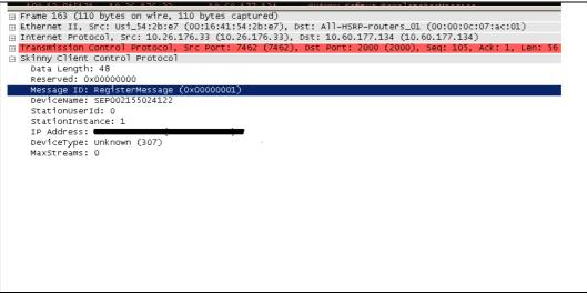
Figure 6: Example of a SKINNY protocol register message
