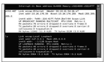
Figure 4: New virtual network interface created for VLAN connection in Linux
