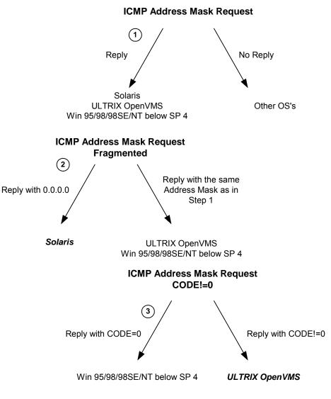
Diagram 2: Finger Printing Using ICMP Address Mask Requests
