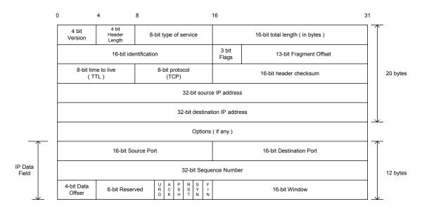
Figure 7: An Example: A TCP packet fragmented after only 12 bytes of TCP information
