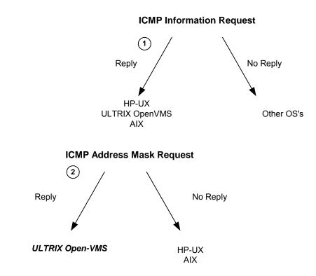
Diagram 3: Finger Printing Using ICMP Information Request Combines with ICMP Address Mask Request
