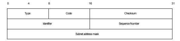
Figure 5: ICMP Address Mask Request & Reply message format
