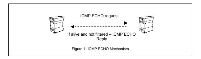
This mechanism is used by the Ping command to determine if a destination host is reachable.
