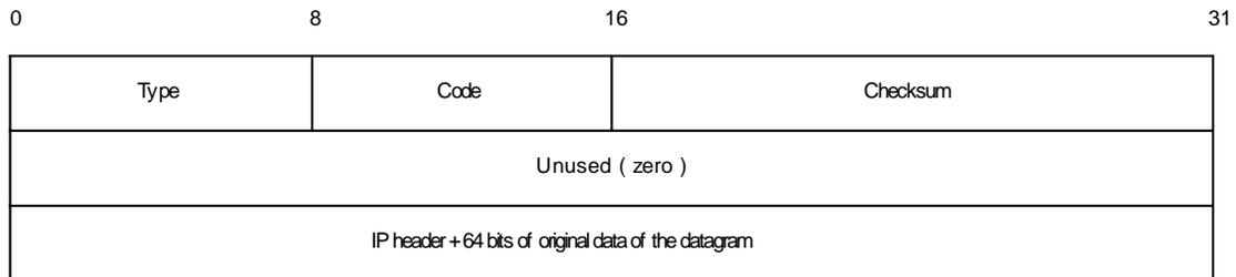
Figure 7: ICMP Time Exceeded message format
