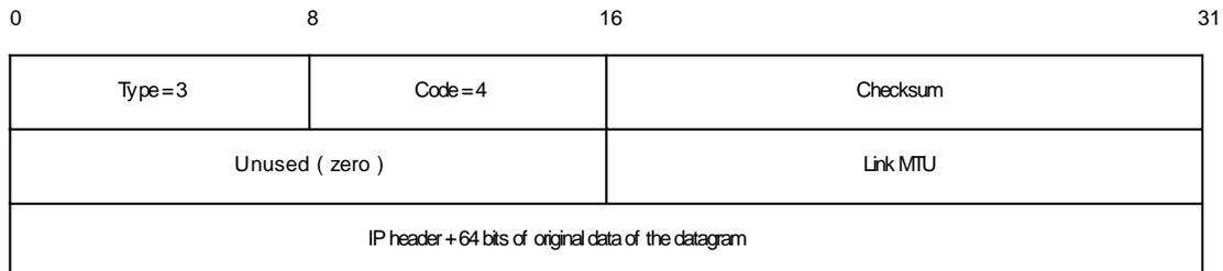
Figure 11: ICMP Fragmentation Required with Link MTU
