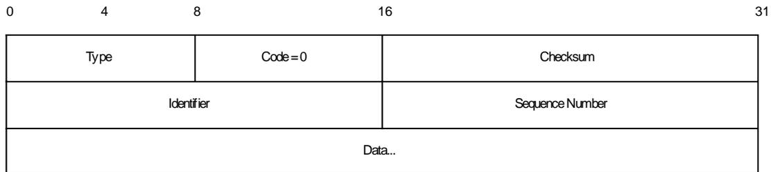
Figure 8: ICMP ECHO Request & Reply message format
