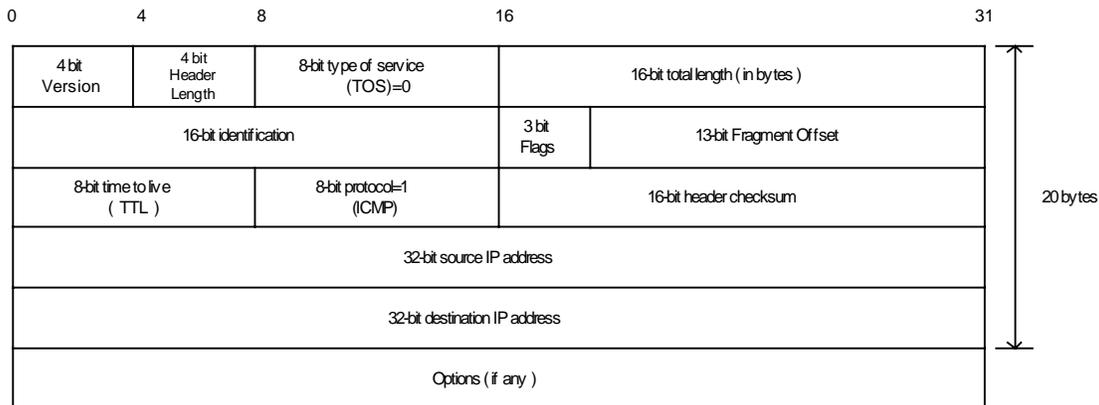
Figure 5: The IP Header
