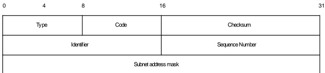
Figure 4: ICMP Address Mask Request & Reply message format
