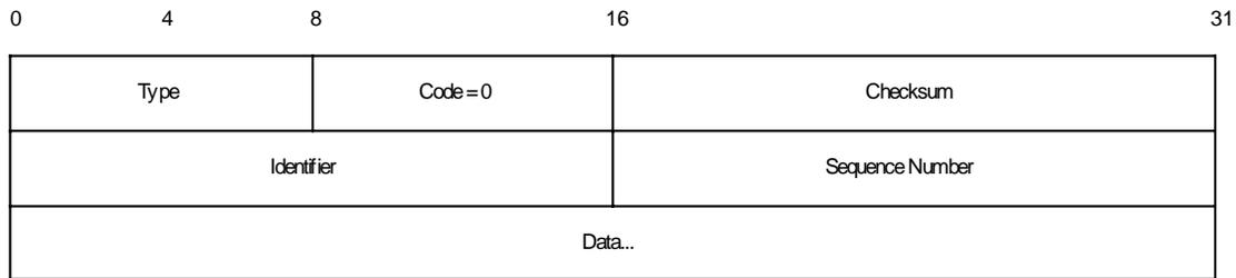
Figure 2: ICMP ECHO Request & Reply message format
