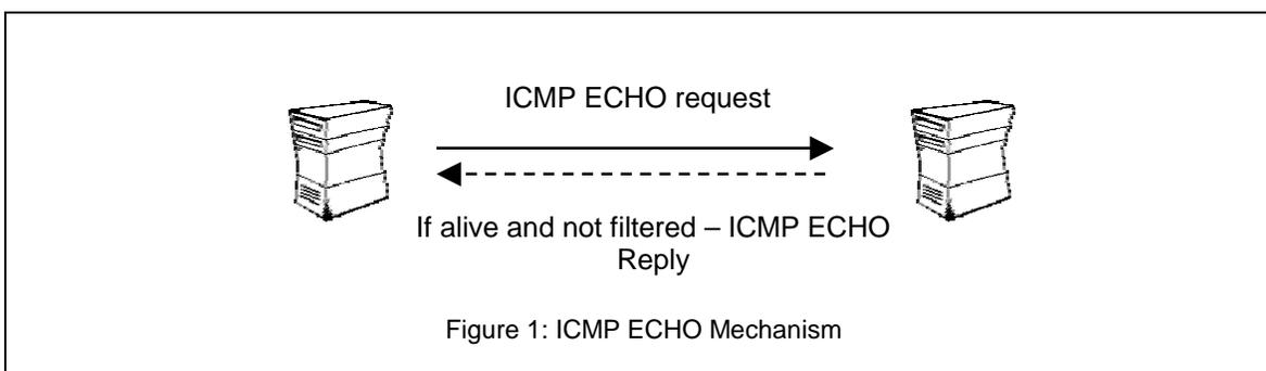
This mechanism is used by the Ping command to determine if a destination host is reachable.
