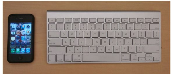
Figure 1: Our experimental placement of a mobile phone running a malicious application attempting to recover text entered using the nearby keyboard.
