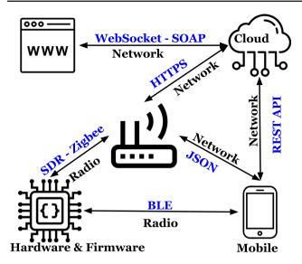
Fig. 2 Architecture mapping
