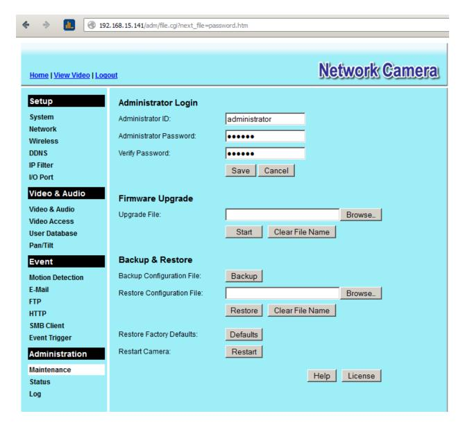
Here the interface of the ip camera so that we can browse the .bin firmware file and upgrade the camera firmware.
