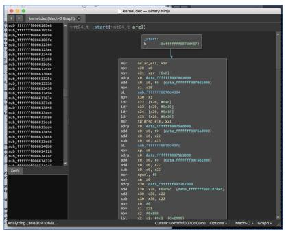
Figure 10 – Disassembling the kernel with Binary Ninja
