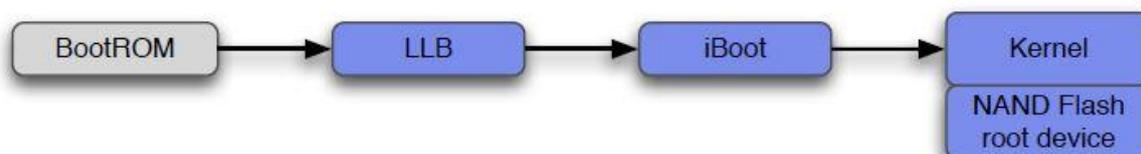
The BootRom is Read only memory (ROM) and it is the first stage of booting an iOS device. BootRom contains all the root certificates to signature check the next stage.
