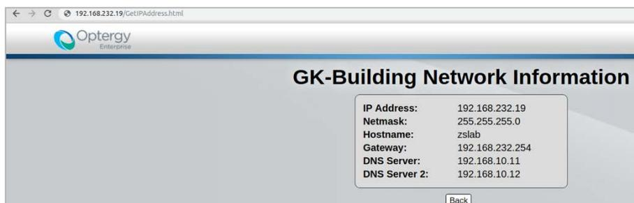
Figure 54. Internal network information disclosure example
