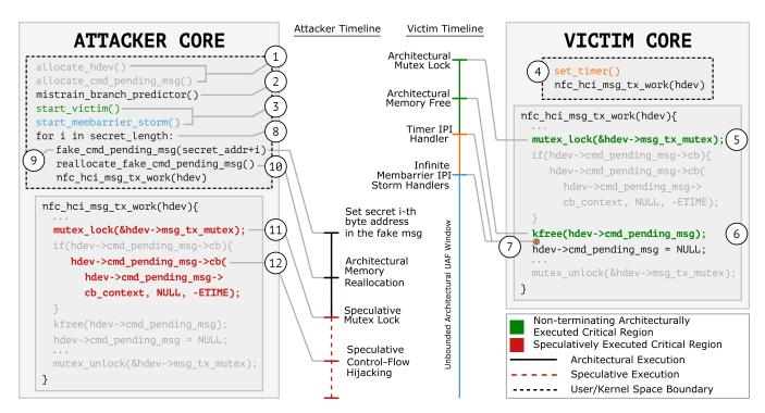
Figure 8: Speculative information disclosure attack exploiting a speculative race condition. Steps 1-4 and 8-10 run in user mode, issuing syscalls to trigger the relevant kernel code. The other steps run in kernel mode. The nfc\_hci\_msg\_tx\_work gadget code is shown only to explain how the speculative race condition is created.
