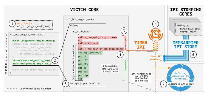
Figure 4: From eight instructions-wide to **unbounded** architectural Use-After-Free exploitation window. Steps 1 and 6 run in user mode, issuing syscalls to trigger the relevant kernel code. The other steps run in kernel mode.
