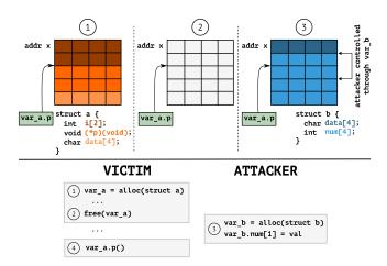
Figure 2: Object reallocation in a UAF attack. First, the victim allocates a heap object which is subsequently freed (steps I and 2). Then, the attacker forces the allocation of an object  $(var\_b)$  reusing memory slot of the victim's object, taking control of the data referenced by the dangling pointer (step 3). Finally, the dangling pointer is dereferenced, ultimately allowing the attacker to hijack control flow (step 4).
