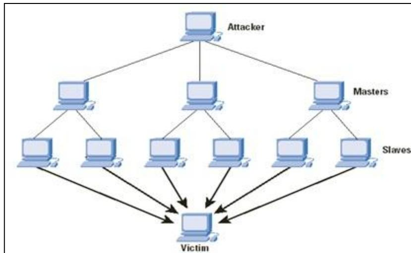
Figure 2: Master Slave architecture in a BOTNET
