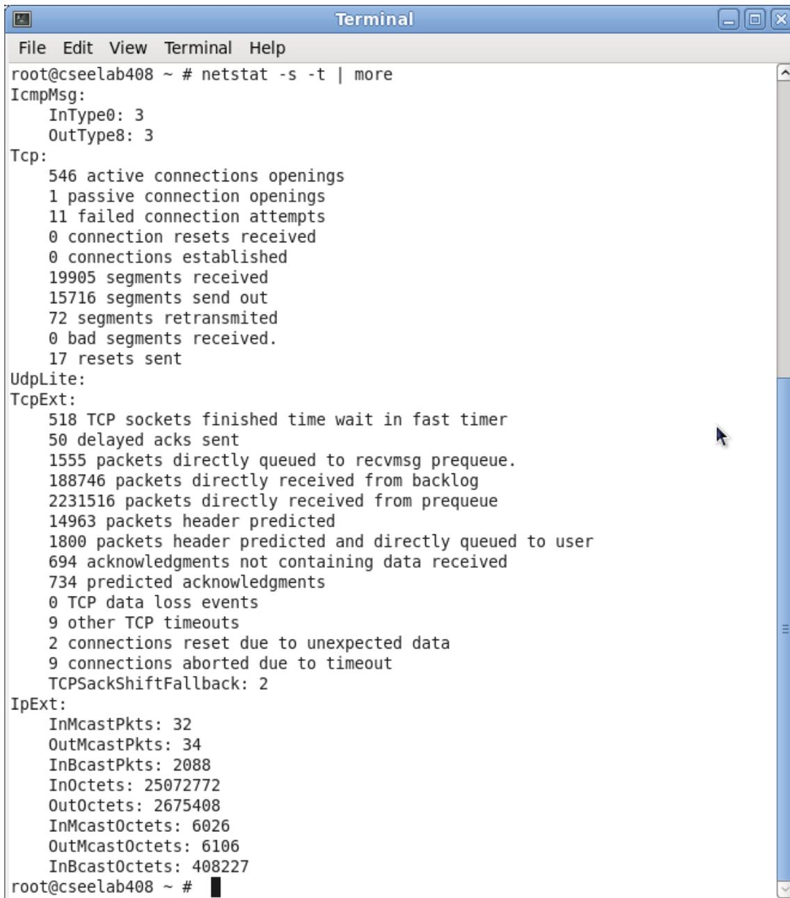
A terminal window titled "Terminal" with a menu bar (File, Edit, View, Terminal, Help). The command executed is "netstat -s -t | more". The output shows statistics for ICMP, TCP, UDP, and IP. ICMP shows 3 received and 3 sent. TCP shows 546 active connections, 19905 segments received, and 15716 segments sent. UDP shows 518 sockets finished time wait. IP shows 32 multicast and 2088 broadcast packets received.
