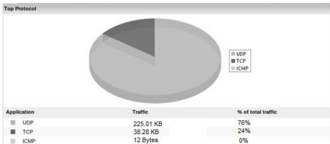
Figure 11: Netflow graph during combined UDP/TCP attack
