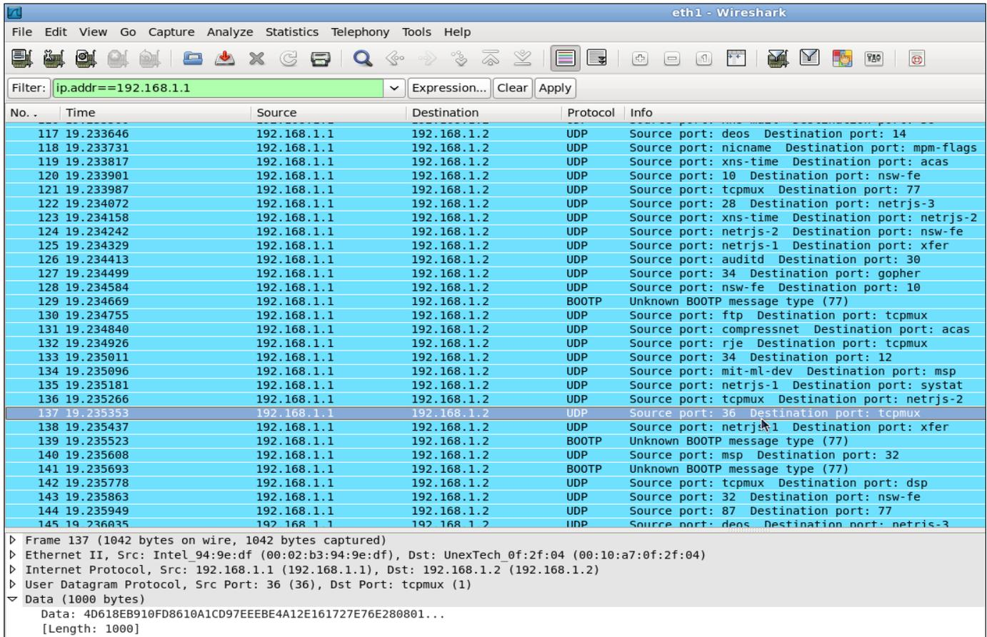
Figure 7: Screenshot of Wireshark during UDP flood attack
