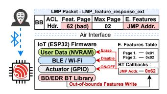
Figure 3: An Illustration of CVE-2021-28138.
