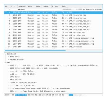
Figure 5: Active BR/EDR Sniffing of piconet. The sniffer captures Baseband + FHS and LMP frames.
