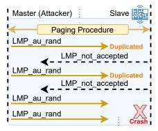
Figure 17: LMP AU Rand Flooding
