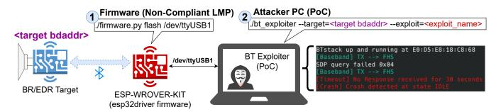
Figure 2: An Illustration of BRAKTOOTH attack scenario
