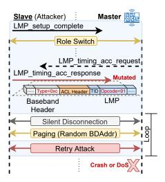
Figure 20: Invalid Timing Accuracy
