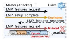
Figure 14: Invalid Setup Complete
