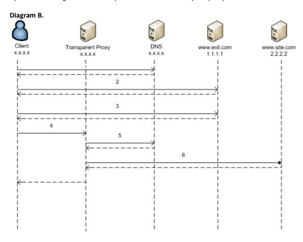
**Diagram B** visualizes the following attack flow when a transparent proxy using Approach B is located between a client and an evil website. The preface for this would be a user visiting a malicious website, or a website with malicious ad which spawns an iframe to an attacker controlled destination.
