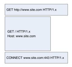
An intercepting transparent proxy receives this request from the client. Upon further inspection it identifies <a href="https://www.site.com">www.site.com</a> in the HTTP request URI or Host header as the end destination host.
