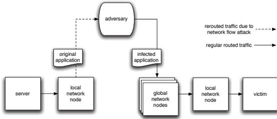
Figure 1: Malicious network node is inserted into the network link using a network flow redirection attack.
