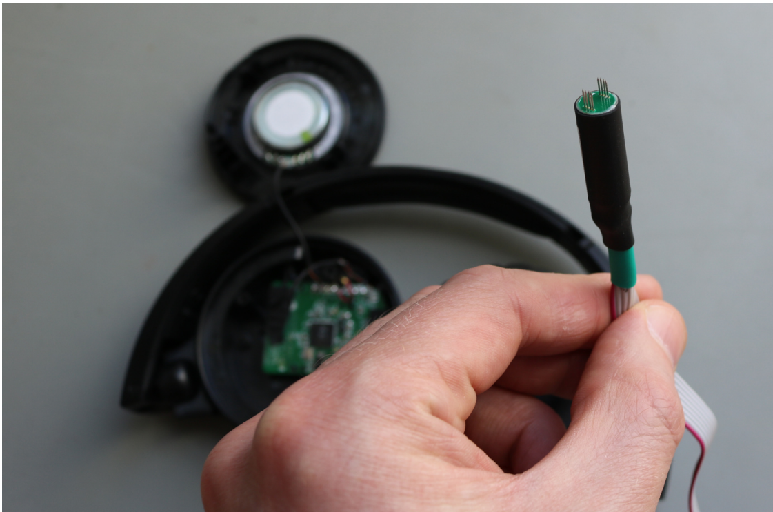
Figure 7: TSSOP-8 adapter used for in-circuit reading of the SPI serial flash
