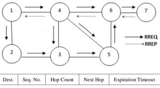
Figure 1. Working and Routing Table of AODV
