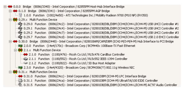
Figure 1: The logical representation of a typical PCI bus
