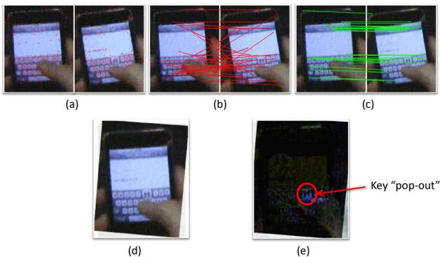
Figure 4: Automatic phone stabilization of two video frames.
