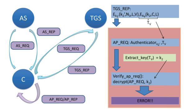
Figure 5: The login process in MIT Kerberos
