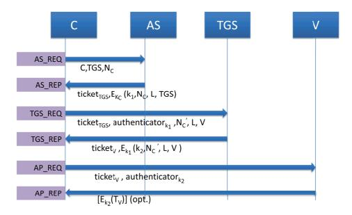
Figure 1: The Kerberos V protocol
