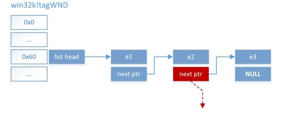
This code gives us a very useful primitive and basically allows us to overwrite 8 consecutive NUL bytes at an arbitrary address in memory with a kernel address. Although we don't directly control the value written and we have the additional constraint that we only can overwrite NUL bytes we will see that this is enough to successfully exploit the vulnerability on Windows 8.1.
