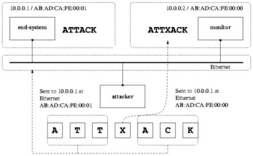
Figure 10: Insertion Attacks at the Link Layer
