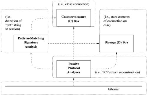
Figure 3: CIDF model of a network IDS
