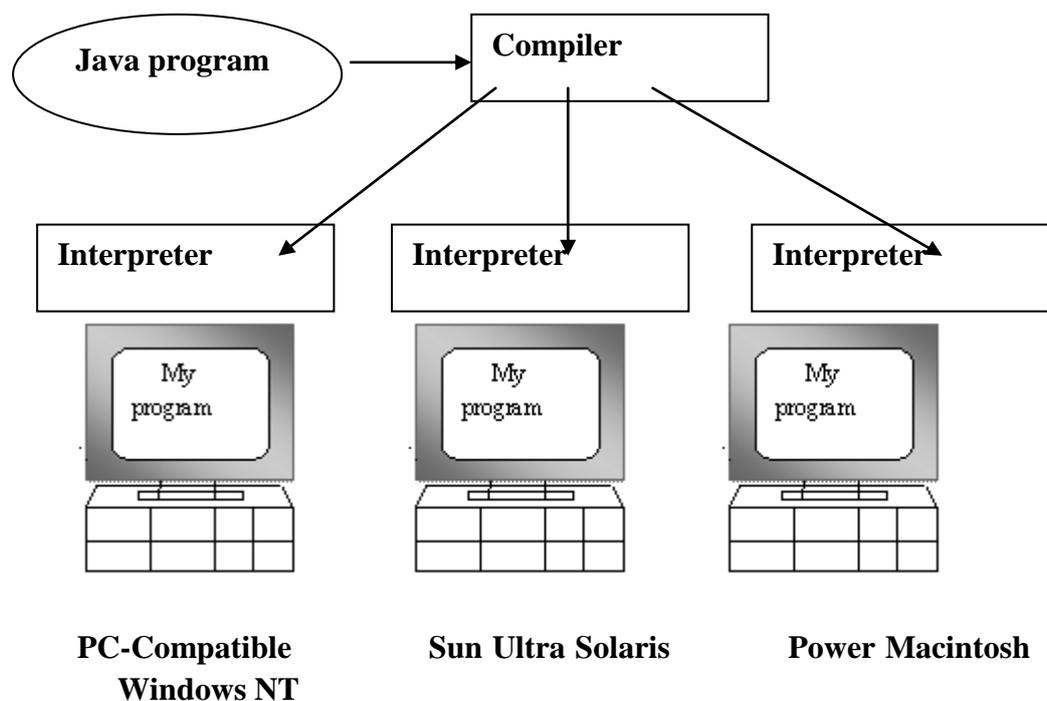
You've already been introduced to the JVM. It's the base for the Java platform and is ported onto various hardware-based platforms.
