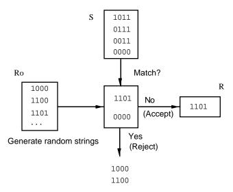
Figure 1: Constructing a set of detectors R for a set of self strings S, using generateand-test. The matching rule used here is "rcontiguous-bits" with r=2. The strings in  $R_0$ are generated at random. The ones that match any of the strings in S are rejected.
