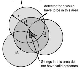
Figure 3: if self strings are presented as points in a plane and the matching rule is Euclidean distance, three self strings  $s_1$ ,  $s_2$ ,  $s_3$  may induce a hole *h* for which no valid detector can be generated.
