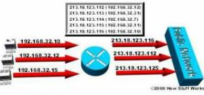
In dynamic NAT, the computer with the IP address of 192.168.32.10 will translate to the first available address in the range from 213.18.123.100 to 213.18.123.150.
