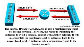
The internal network is usually a **LAN** (**Local Area Network**), commonly referred to as the **stub domain**. A stub domain is a LAN that uses IP addresses internally. Most of the network traffic in a stub domain is local, it doesn't travel off the internal network. A stub domain can include both registered and unregistered IP addresses. Of course, any computers that use unregistered IP addresses must use Network Address Translation to communicate with the rest of the world.
