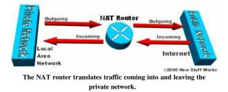
This is where NAT (<u>RFC 1631</u>) comes to the rescue. Basically, Network Address Translation allows a single device, such as a router, to act as agent between the Internet (or "public network") and a local (or "private") network. This means that only a single unique IP address is required to represent an entire group of computers to anything outside their network.
