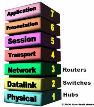
NAT operates at the Network layer (Layer 3) of the OSI Reference Model which makes sense since this is the layer that routers work at.
