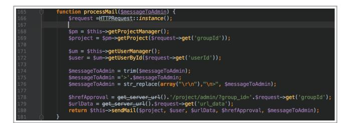
The main problem is Line 172. Tuleap is creating \$user variable through user input that shipped with **userId** HTTP POST parameter. That means we can change userId with another userId that doesn't represent us at all. This parameter must be taken from SESSION instead of HTTP request.
