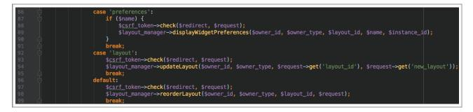
Line 94 will be executed when user input **action** is layout. **updateLayout()** function which belongs to LayoutManager class takes 5 different function parameters.
