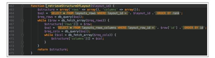
Bingo..! \$layout\_id is used during sql query building without PDO nor escaping.It is a time-based sql injection vulnerability.
