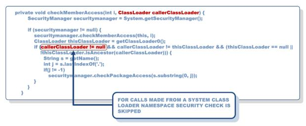
Figure 10. Implementation of checkMemberAccess() method.
