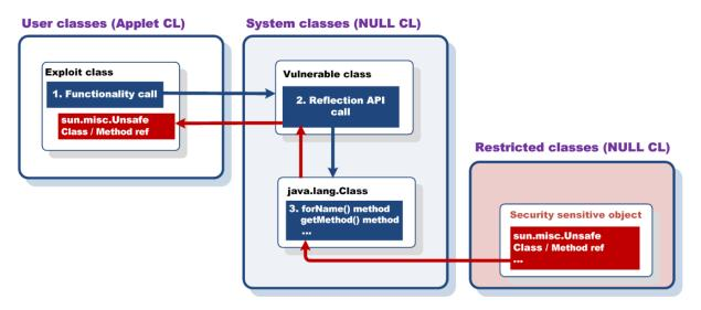
Figure 11. Generic idea behind the abuse of Reflection API calls used by system classes.
