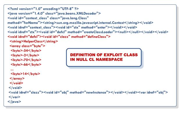
Figure 23. XML Message breaking Java 7 security sandbox.
