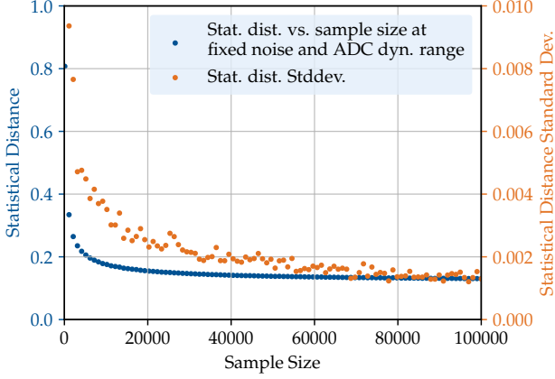
FIG. 3. Simulated Statistical distance and its standard deviation at a fixed noise value of 1.5 % and an assumed ADC dynamic range fraction of 50 %. With increasing sample size, both values decrease and converge. This emphasizes that simulations have to match the experimental conditions.
