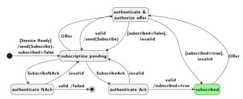
Fig. B.2. State machine for SOME/IP subscription handling with authentication and authorization at the client side not including, retransmissions, and timeout handling.
