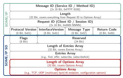
Fig. A.1. SOME/IP message layout for service discovery messages [13].
