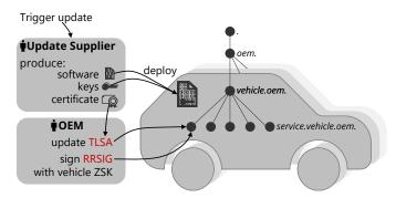
Fig. 1. Distributed and secure credential management for automotive services based on the DNSSEC ecosystem that decouples the software signing by the update supplier from the record signing by the OEM.
