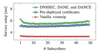
Fig. 4. Mean subscription setup time in a synthetic study for 1 publisher with 1 to 50 subscribers across the implementations.
