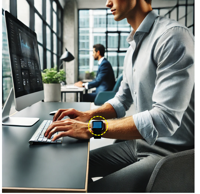
Fig. 1. Illustration of the attack model. A programmer working in front of a highly secure or air-gapped computer wears a smartwatch on their wrist. The infected computer transmits sensitive data, such as keylogging information, modulated onto ultrasonic signals, which are covertly received by the smartwatch.
