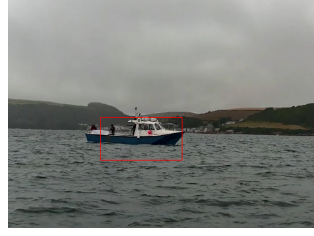
(b) Radar contact transformed into the optical coordinate space using the homography mapping. Projection is shown as a red bounding box.
