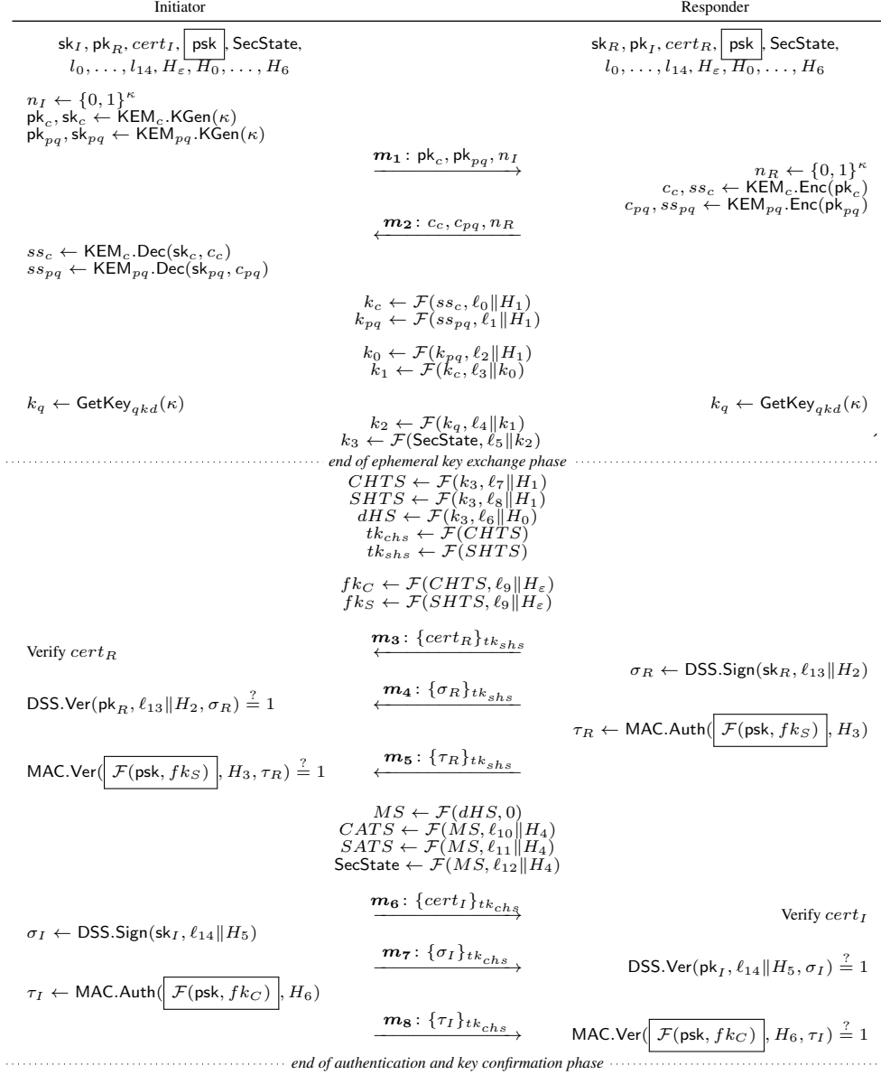
Fig. 2: One stage of the VMuckle protocol with a classical KEM \text{KEM}_c , a post-quantum KEM \text{KEM}_{pq} , a MAC \text{MAC} and a PRF \mathcal{F} , where k_q is a symmetric QKD key (provided out-of-band via the function \text{GetKey}_{qkd} ), and \text{psk} is a pre-shared key. cert_I and cert_R are certificates (provided out-of-band) for the public keys pk_I and pk_R , respectively. CATS and SATS are the client and server application traffic secrets, respectively. Messages m_i: \{m_{i,1}, \dots\}_k denote that m_{i,1}, \dots are encrypted with an authenticated encryption scheme using the secret key k . The various contexts and labels are provided in Tables I and II. In the first run, \text{SecState} is initialized as an empty string \perp . Changes to Muckle+ are denoted \boxed{\phantom{x}} .
