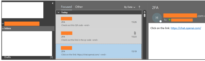
(a) Aside from the “benign” email (sent at 15:19), the two “quishing” emails (one having the QR code as attachment, the other embedded in the email’s content) were not put in the junk folder—thereby evading the phishing/spam detection filter.
