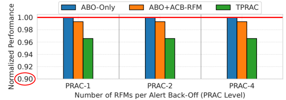
Figure 11: Performance comparison of TPRAC and insecure baselines, ABO-Only and ABO+ACB-RFM, across different PRAC levels at a RowHammer threshold of 1024. Performance remains consistent across PRAC levels. TPRAC and ABO+ACB-RFM incur slowdowns of 3.4% and 0.7%, respectively, due to proactive RFMs reducing DRAM bandwidth. In contrast, ABO-Only shows almost no overhead, as ABO-RFMs are rare in benign applications at this threshold.
