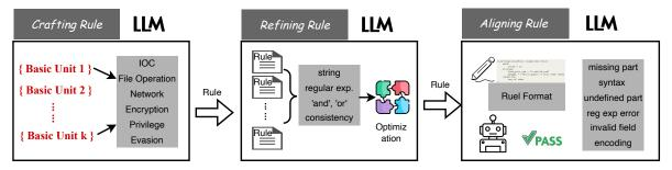
Fig. 3: RULELLM: the architecture of the LLM-based rule generation: (1) crafting basic-unit rules, (2) refining rules, and (3) aligning rules.
