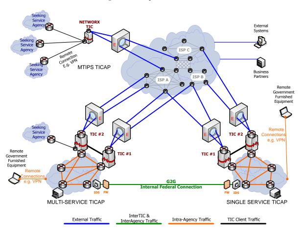
Figure 2: Conceptual TIC Architecture
