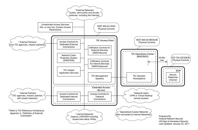
Figure 7: TIC Access Point Functional Block Diagram<sup>2</sup>
