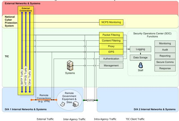
**Figure 4: External Connection Security Pattern**
