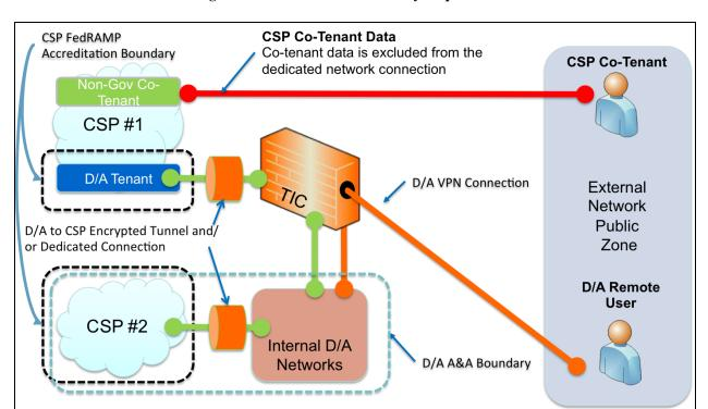
Figure 16: D/A-to-CSP Connectivity Requirements
