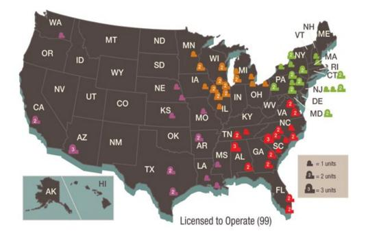
Figure 1. U.S. Operating Commercial Nuclear Power Reactors
