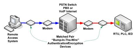
Figure 4. Bump-in-the-wire installation.
