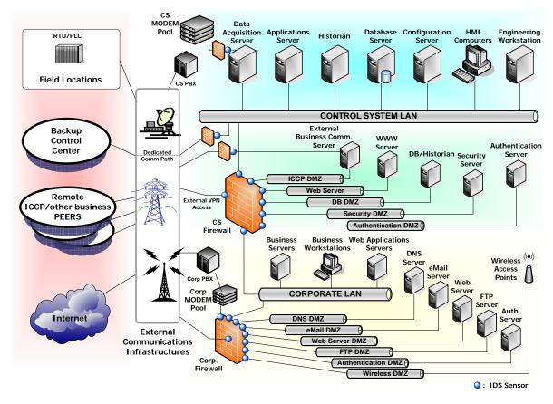
DHS Recommended Network Architecture Design for Control System Security.<sup>h</sup>
