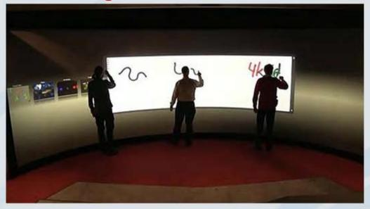
It's gigantic ! It can handle simultaneous over 100 touch points! It has a curvature of 135 degrees! And best of all, it is NOT the newest, insanely expensive gadget to hit the market. Instead, this touchscreen was hacked together with bunch of PCs, video cameras, projectors and cheap infrared illuminators at the University of Groningen, in the Netherlands.
