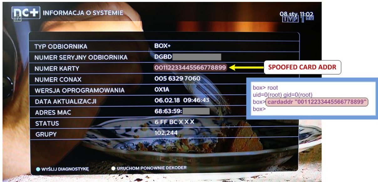
Fig. 26 Spoofing STBs smart card address.
