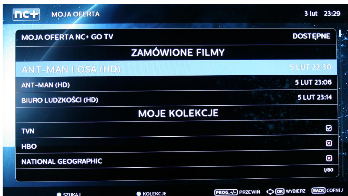
Fig. 36 STB screen indicating successful VOD orders conducted through JSON API and arbitrary price input.
