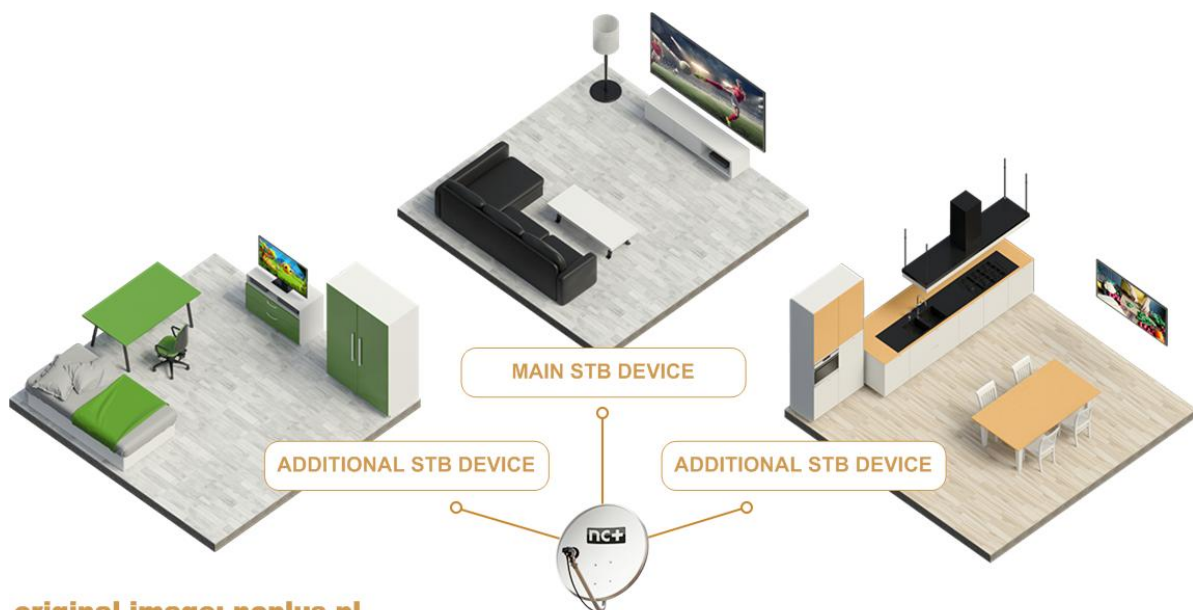
Fig. 9 Schema of a sample Multiroom installation.
